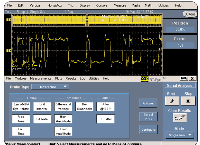
Figure 25. The user interface window of a serial analysis tool running on a real-time oscilloscope.
